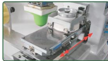
Platform in / out movement (Pad clean underneath)
