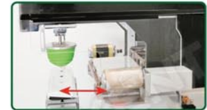
Pad in/out stroke for max. throat depth
