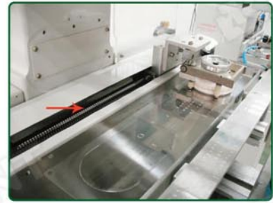
Lead-screw work platform
