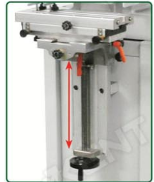
User-friendly: Steering up/down work table
