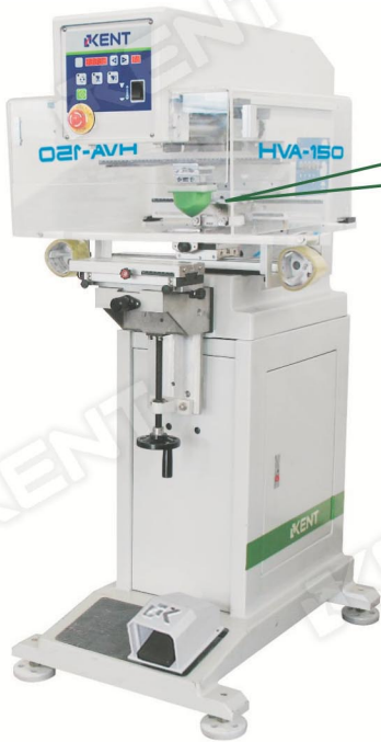
AVC - Automatic Viscosity Control (patented)
