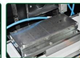
Vacuum platform (Absolute flatness for high quality requirement)
