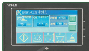
PLC control touch screen panel
