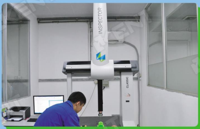
三坐标3D胶头测量角度/弧度 CMM (Coordinate Measuring Machine) 3D measurement
